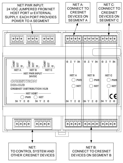
Hardware Connections for the DIN-HUB
